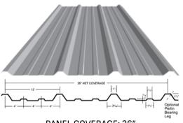
PANEL COVERAGE: 36" RIB HEIGHT: 1 1/4" **RIB FEATURES: 12" CENTERS GAUGE: 26 GA, 24 GA**
